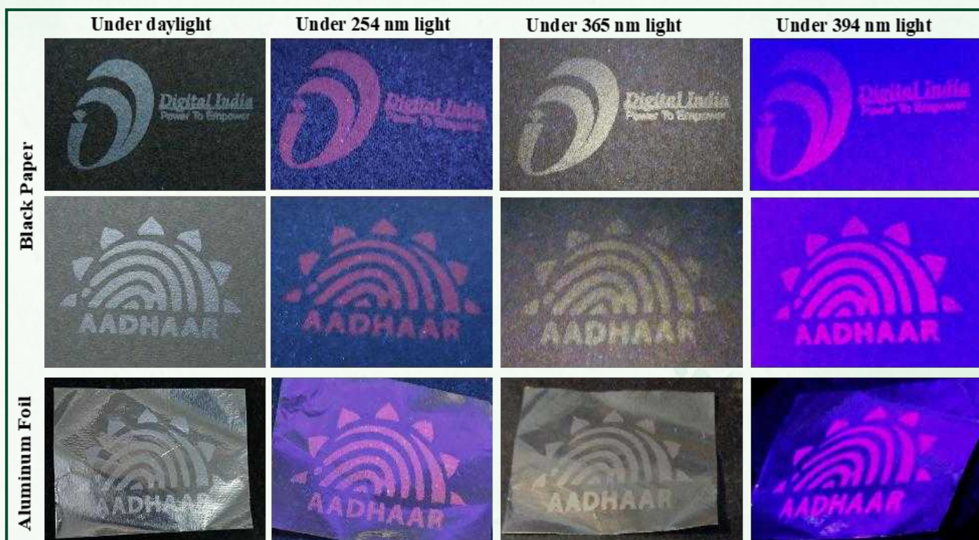
Figure. Digital images of anti-counterfeiting patterns on black paper and aluminum foil under daylight, 254, 365, and 394 nm UV light.
