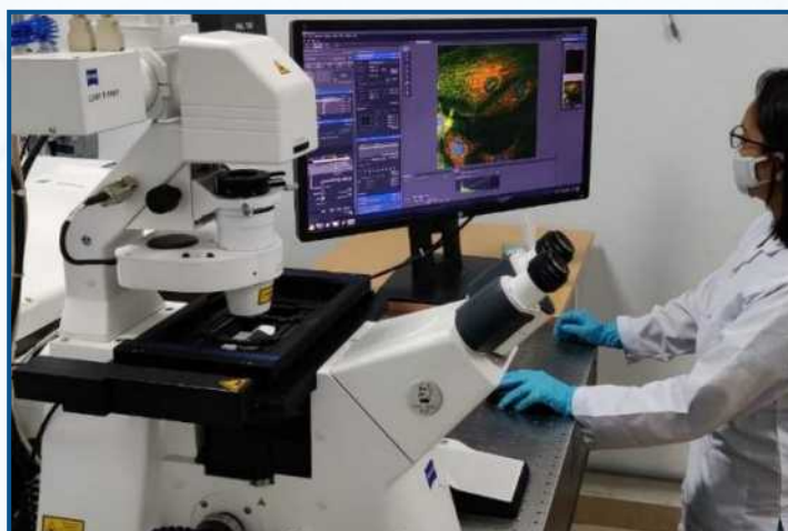
Laser scanning Confocal Microscopy with AIRY scan mediated Super resolution model
