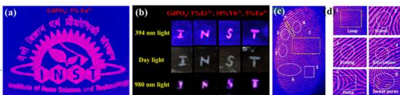
Figure: (a) Photograph of INST logo printed with \text{Eu}^{3+} doped \text{GdPO}_4 under 394 nm light, (b) INST letters written with \text{Eu}^{3+} , \text{Er}^{3+} , \text{Yb}^{3+} doped \text{GdPO}_4 under day light, 394 and 980 nm light, (c) fingerprint developed under 394 nm light (d) enlarged regions of fingerprint.
